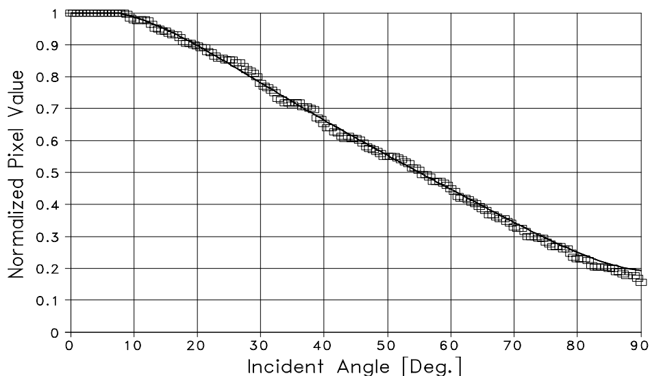
Figure A.5 Off-Axis Luminance Transfer Function at f/4
