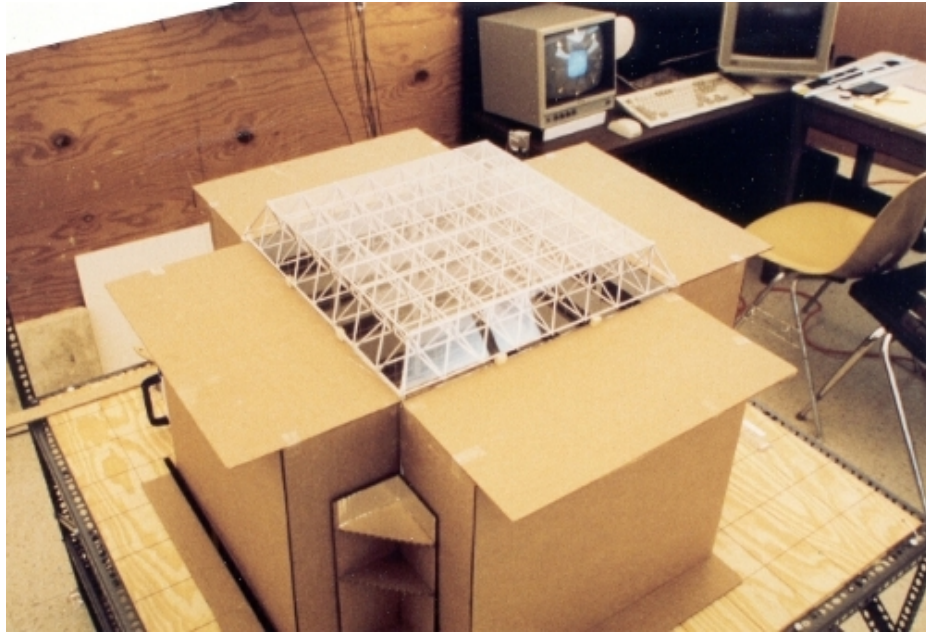
Figure 8.34 Photo of Flat Horizontal Skylight Installed on Kleberg Atrium Building Scale Model
