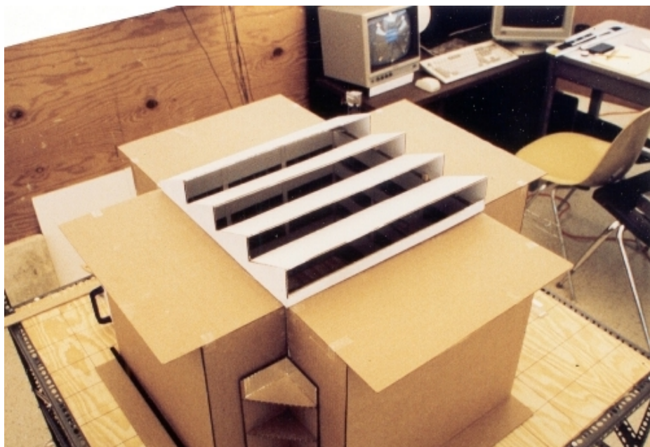
Figure 8.33 Photo of 4-Unit Sawtooth Canopy Installed on Kleberg Atrium Building Scale Model
