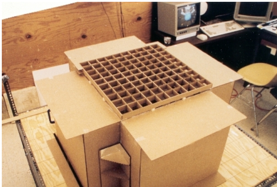
Figure 8.37 Photo of Waffle Skylight Installed on Kleberg Atrium Building Scale Model
