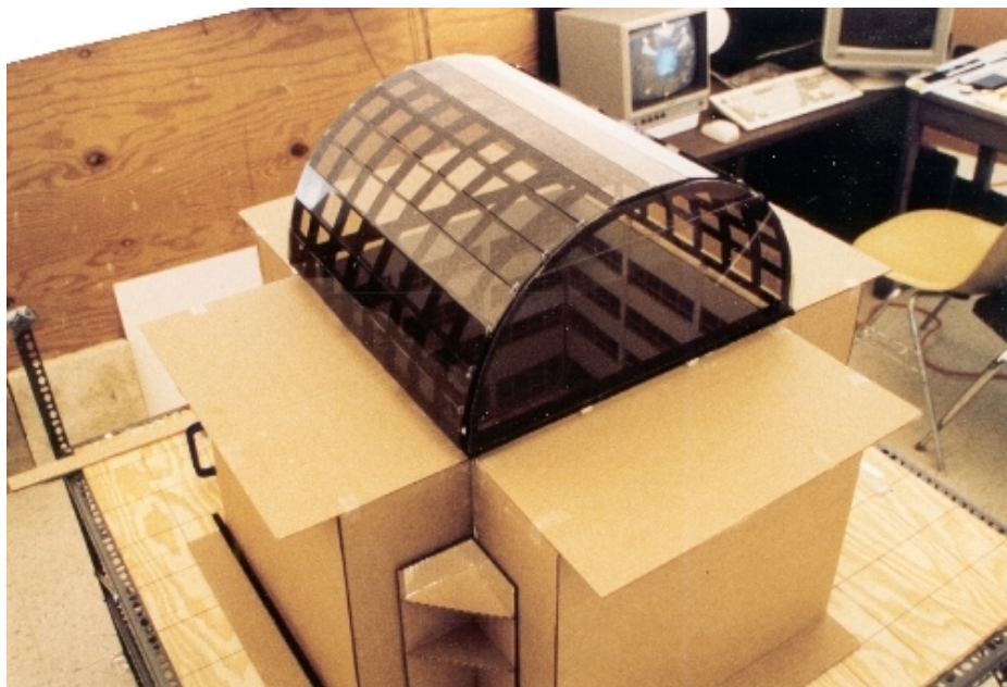
Figure 8.35 Photo of Barrel Vault Skylight Installed on Kleberg Atrium Building Scale Model
