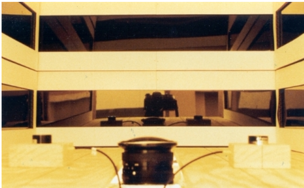
Figure 5.17 Fisheye Lens in Atrium Scale Model
