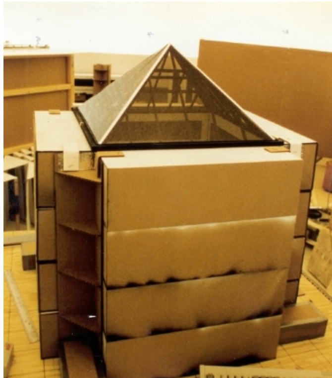
Figure 5.5 Tinted Pyramid Skylight Installed on Atrium Scale Model
