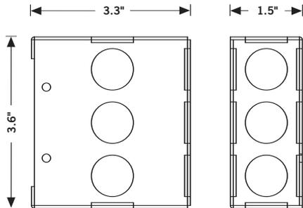
Énergie junction box supplied to allow the fixture to be mounted flush against the wall with no exposed mounting plate.
