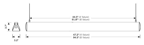
\* 8' fixture has an additional suspension point, located in the center of the fixture
