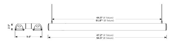
\* 8' fixture has an additional suspension point, located in the center of the fixture
