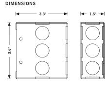
Energie junction box supplied to allow the fixture to be mounted flush against the wall with no exposed mounting plate.
